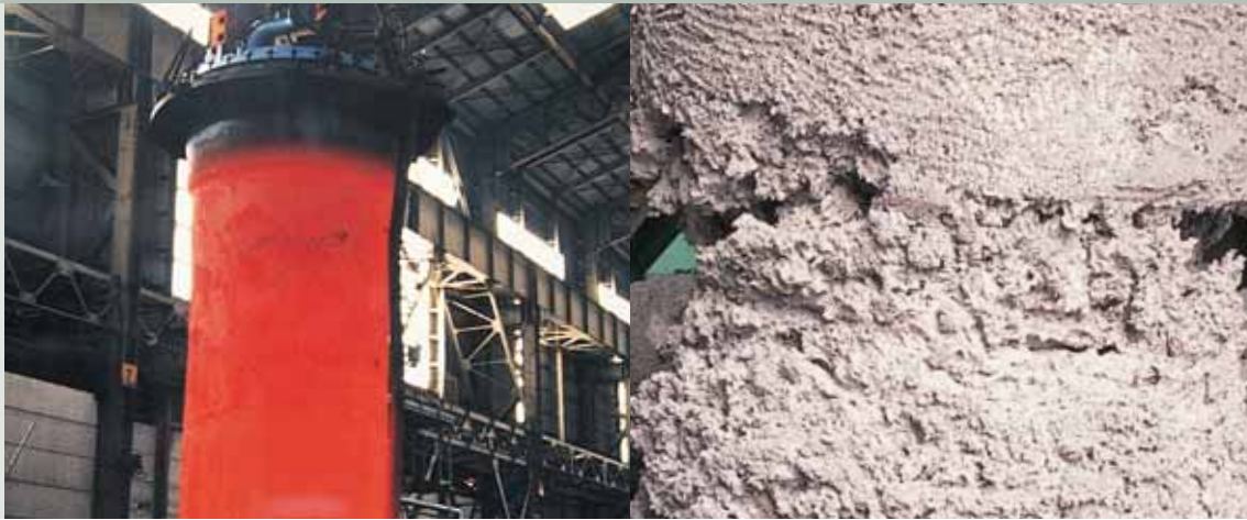
Left: Manufacturing of Titanium Sponge Right: Titanium Sponge
