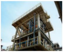
Titanium Tetrachloride Distillation Tower
